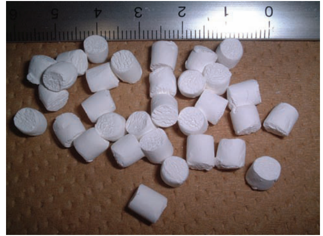
Fig.3: A CO 2 absorbent appearance photograph
