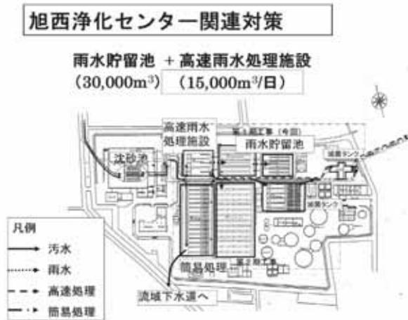
Fig. 4: The plan of combined sewer overflow control target at Kyokusai treatment Plant
