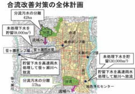
Fig.3: The total plan of combined sewer overflow control target
