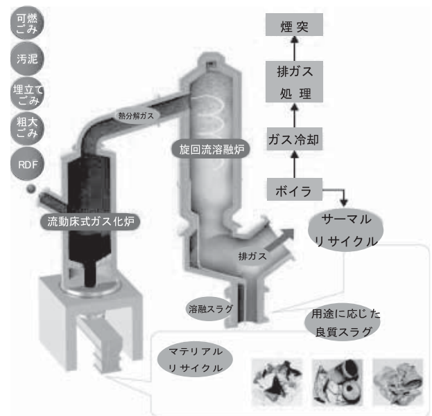
Fig. 1 Outline of Gasification and Melting Process
