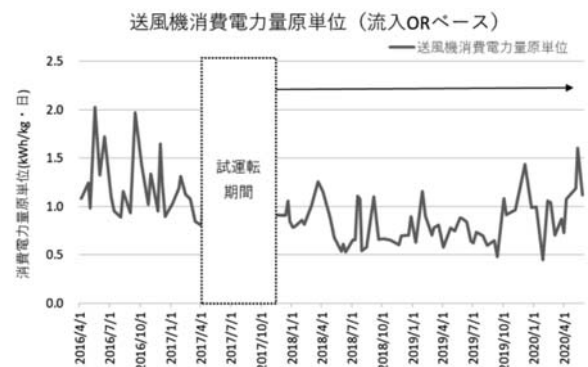
Fig. 8 Time-course change of blower electricity consumption per unit OR
