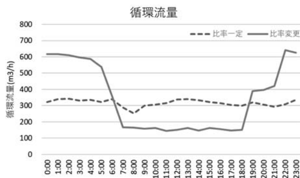
Fig. 9 Operation results of recirculation ratio
