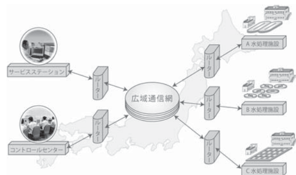
Fig. 3 Wide-area remote management system
