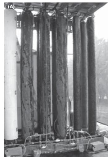
Fig. 3 A picture of the pilot scale microbial fuel cell treating breweries wastewater in Australia<sup>13)</sup>
