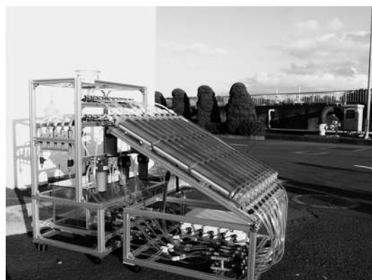
Fig. 4 Test plant of hydrogen generation using sewage sludge
