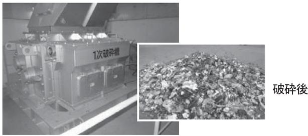
Fig. 5 Primary shredder
