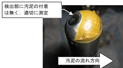
Fig.10: Situation of The Adhesion of Sludge to The Detector (Low Flow Rate, 0.2m/s)
